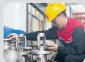
Wall thickness test
